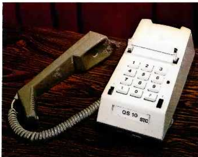
A variation on the theme of the pushbutton telephone is this repertory dialler, which stores up to ten frequently-used numbers and dials them automatically at the push of a button.
